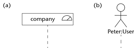
Fig. 8-5 Alternative notation for Lifeline. The fundamental type of represented element is shown as: (a) an icon decoration, (b) a large icon.
